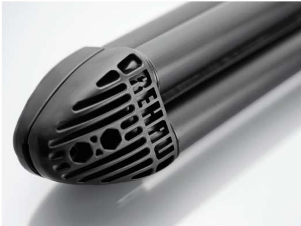
REHAU's new generation of ground-source probes are made of PE-RC, which stands for *Polyethylene Resistant to Crack*. It is defined as an advanced non-cross linked polyethylene, characterised by longer lateral chains compared to PE 100. These create an increased resistance to stress cracking and puncture loads (Full Notch Creep Test > 3,300h). All the other properties of PE-RC are the same as conventional PE 100 (temperature resistance, requirement for welded connections).
