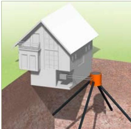
*Coaxial probes for geothermal radial drilling*
